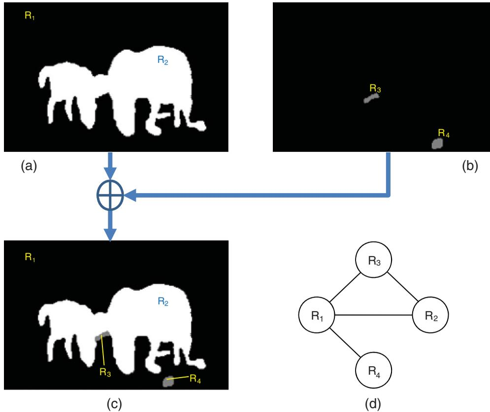
**Fig. 4** Example of a RAG construction: (a) A labeled binary map composed of core candidate region and background region, (b) undefined regions with region labeling, (c) a trimap combined (a) and (b), and (d) a RAG corresponding to (c).
