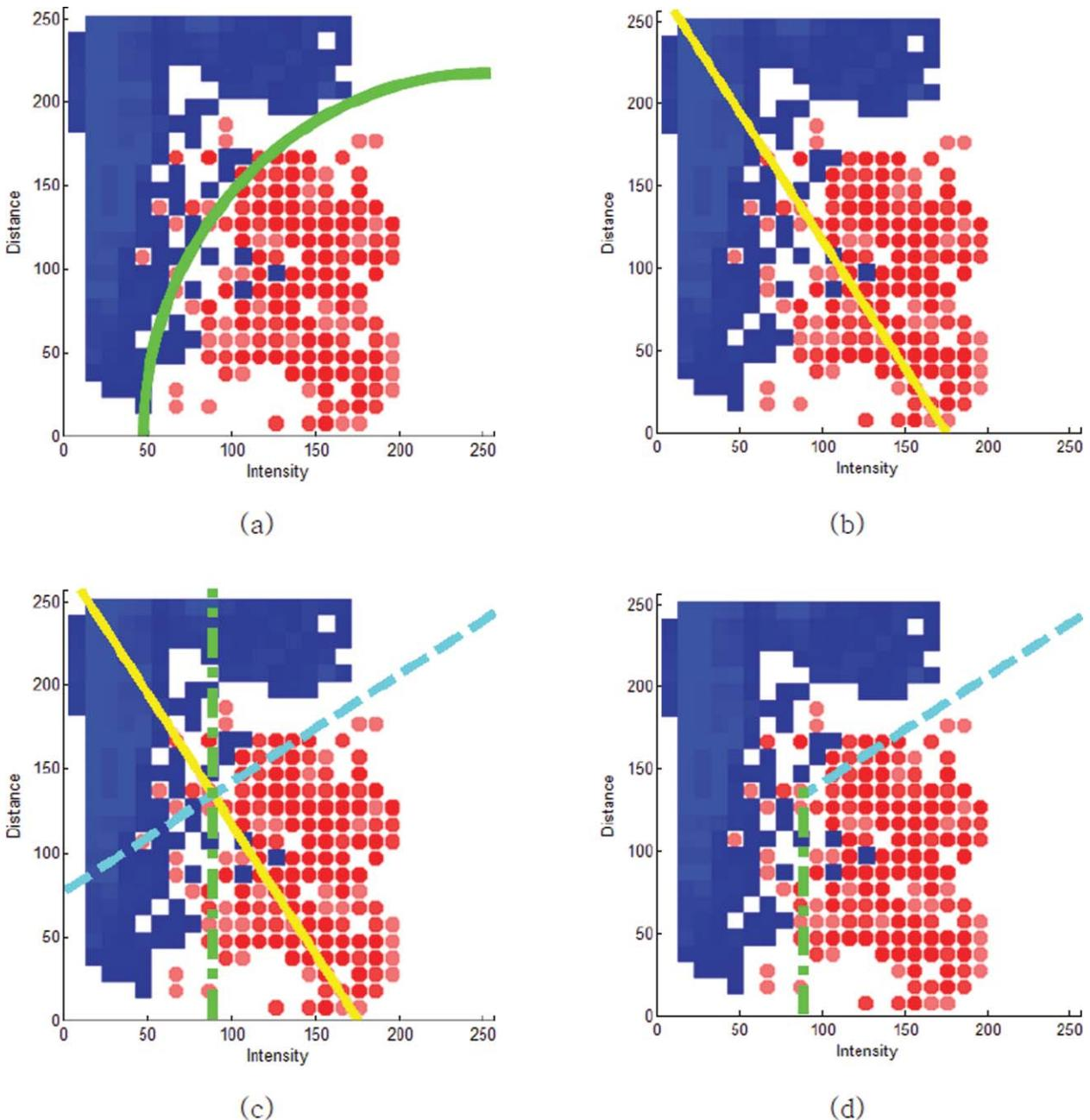
**Fig. 2** (a) The green curve is a manually selected optimal decision curve in the 2-D histogram (intensity-distance domain), (b) line is the principal component axis corresponding to the largest eigen-value by principal component analysis, (c) dashed line, and the dashed-dotted line are decision functions, and (d) the background and the target region. (Color online only.)
