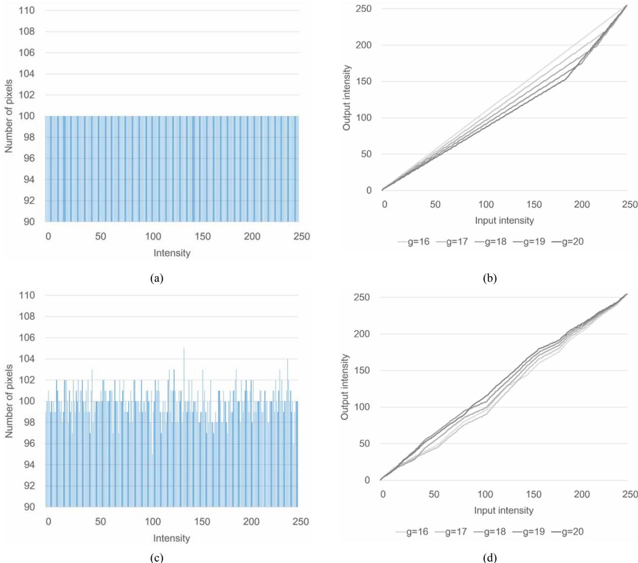
Fig. 1. Transformation functions for each level of the histogram grouping by GLG (a) Uniform histogram, (b) Transformation functions by the grouping of (a), (c) Histogram changed randomly, (d) Transformation functions by the grouping of (c).
