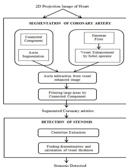
Figure 3: Flow Diagram of Mirunalini's Method [21]
